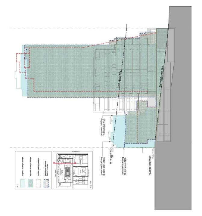
Figure A2 - Building 1 & 3 height compliance plan (existing, approved/commenced and proposed) (Source JPRA)
